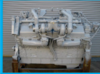
Fire Pump Skid Fitted With 8V92 Engine
