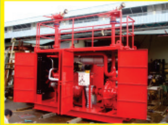
Fire Pump Skid Fitted With 8V92 Engine
