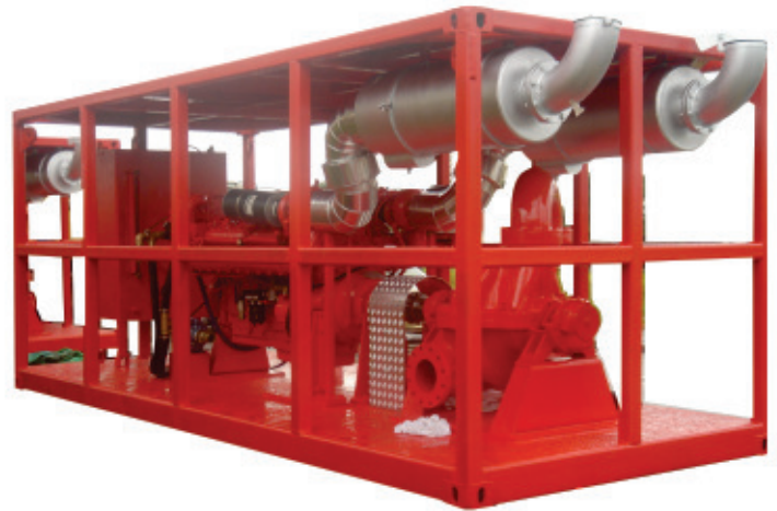
16V92TA Engine c/w Multi-Stage Pump in 20ft Skid (Built to DNV 2.7.1 Offshore Container Standard)
